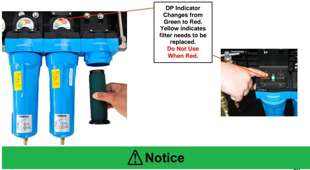
The interior of the Filter Bowls can be cleaned with a diluted solution of Simple Green<sup>™</sup> and flushed thoroughly with clean water. This will assist to prolong the life of the element, bowl, and auto drain.
